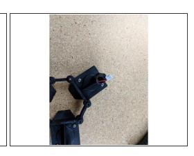
Ne careful in this step not to pull on the blower fan wires as they can be damaged if pulled on.
