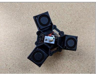
This guide will show you how to assemble the SE300 hot end and effector platform.
