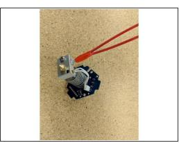
Insert the Thermistor connector into the JST connector on the bottom of the Probe PCB.
