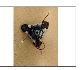
Using the three #4, 1/2" screws, fix the hot end assembly to the effector platform at the locations indicated by the red circles.
