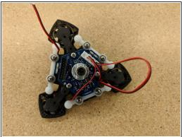
Route the fan leads as shown and plug into the JST connectors at the top of the PCB.
