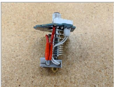
Finally, solder the heater cartridge leads to the Probe PCB.
