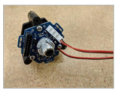
Connect the hot end fan to the JST connector on the far right of the PCB as shown.
