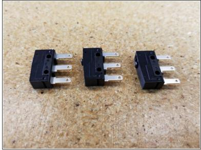
YOUR END STOP SWITCHES COME WITH A SMALL METAL ACTUATING LEVER, CAREFULLY REMOVE IT. IF YOU DON'T REMOVE THIS LEVER, YOUR MACHINE WILL NOT HOME OR WORK CORRECTLY.
