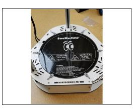
A Be sure to pass the bed wires through the black injection molded insulator BEFORE soldering the wires to the bed!
