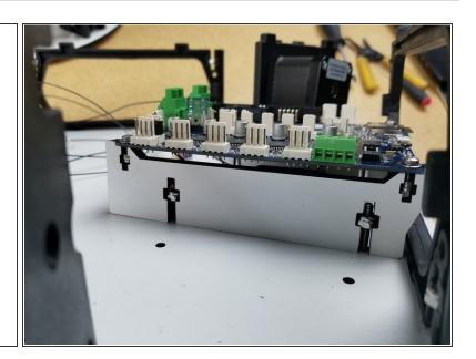
Install the Duet as shown, using the M3 10mm screws and M3 nylon lock nuts.
