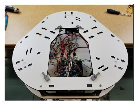
Install the top plate the same way the other main frame plates have been installed, using the 6/32 1" bolts and captive nylon lock nuts in the motor and side panel plastics.
