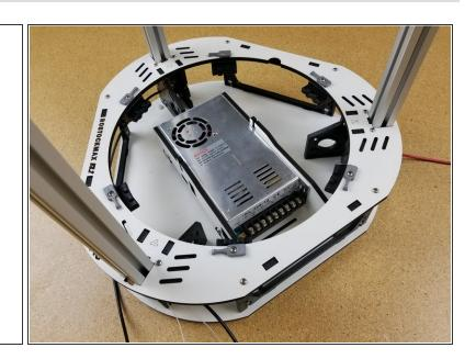
You will now install the remaining two towers just as you did the Z tower. Begin with the Y tower, which has the white thermistor wires run through the center hole.
