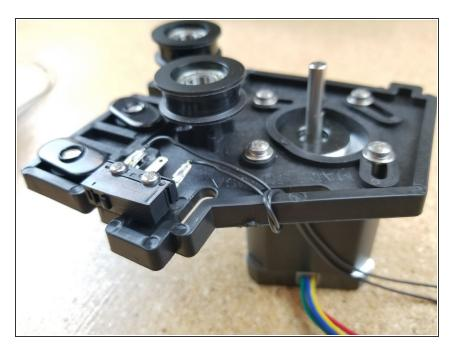
This is not required, but looping the wires through this plate will act as a strain relief and help manage the wires.
