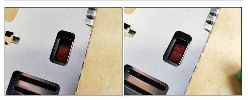
⚠ If you are located in the US, make sure the 220/110 switch is in the 110 (115) position, as indicated by the arrow. This defines the input voltage the power supply expects.
