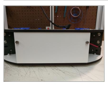
You can now install the remaining side covers with 10-32 socket head cap screws.
