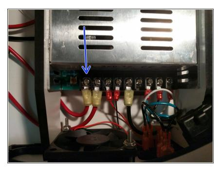
The 700mm long 12awg red wire that you previously crimped the ring terminal on should now be connected to the power supply in the location indicated by an arrow. Route the wire under the PSU blocker with other red 12awg wire.
