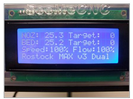
When the firmware has successfully been installed you will see the printer name on the main screen has changed and is now: PrinterModel Dual
