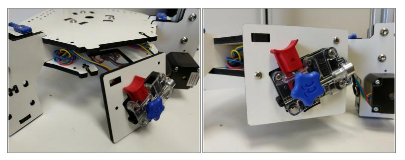
• Install the EZR Struder using the (2) 6-32 X 1" machine screws. You can fully tighten these.
