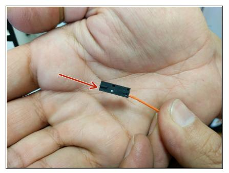
Insert the prepared wire and connector in the 2 pin latching connector in pin 1 (indicated with an arrow until you hear / feel a click. (just like with the end-stop wires)
