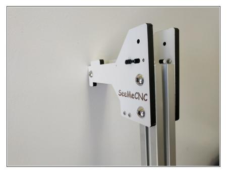
Slide the top tower mount assembly onto the 24" long piece of TSLOT until it reaches the stop screws.
