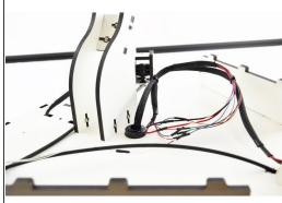
Tame any excess wires in the top of the printer with cable ties.
