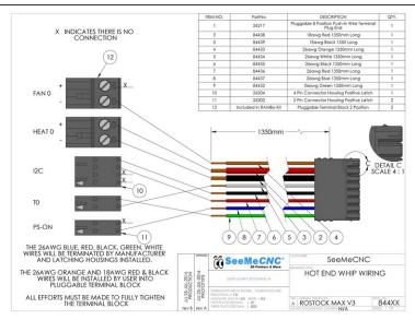
Use the image to the left to perform a final check of your wiring connections. All connections are outlined, and these connections must be made in order for the printer to be functional with the HE280 Hotend.
