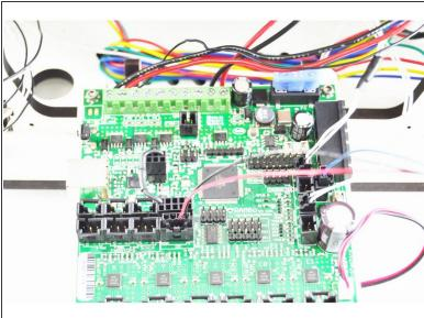
Plug the I2C wires (4 pin latching housing) into the RAMBo board in the I2C location. This
