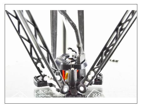
Plug the 8 position plug into the top of the hotend. This plug is keyed on two corners so pay particular attention to the orientation and do not force it if it is not going.
