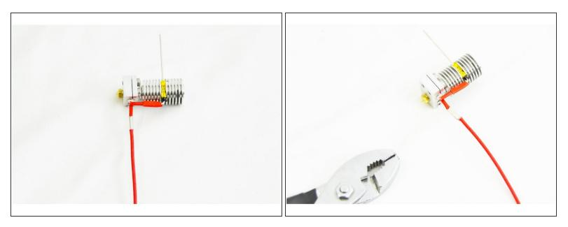
• Slide the High Temp Fiberglass Insulated Wire (side with 10mm stripped, into the other end of the wire ferrule (inserted in the last step)
