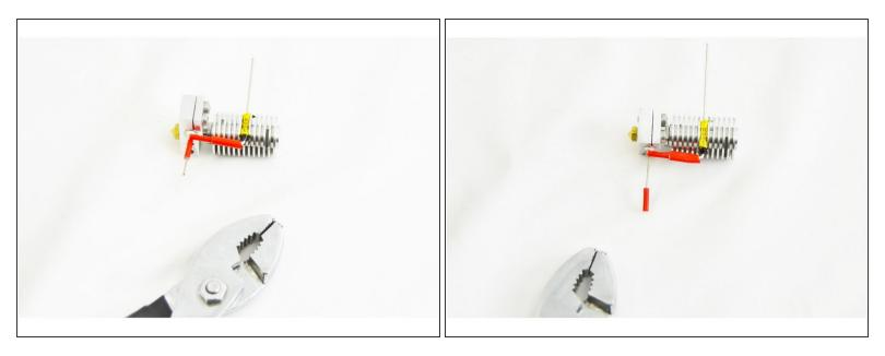
• Use a pair of pliers to crimp the ferrule to the leads. Do this in three steps: roughly locate the midpoint of the ferrule and crimp the upper portion (side with the thermal safety fuse lead), then the lower side (side with the heater cartridge lead), and finally crimp, one last time in the center of the ferrule.
