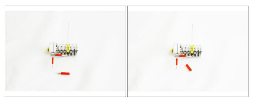
Insert the non-insulated wire ferrule into one of the pieces of red silicone high temp insulation, centering it.
