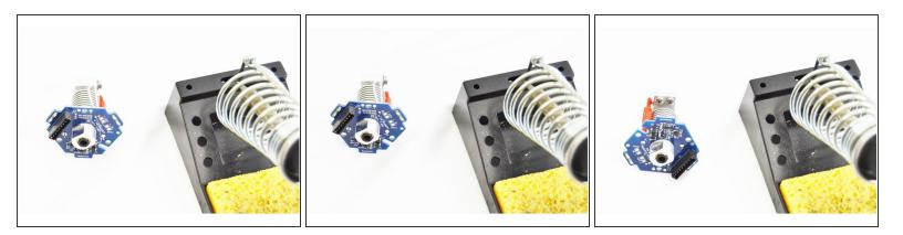
• After the through hole connections have been soldered, trim the excess thermistor leads on the top side of the HE280 Hotend PCB board. These do <u>NOT</u> need to be flush with the board, we just need to ensure that they can not short against each other.
