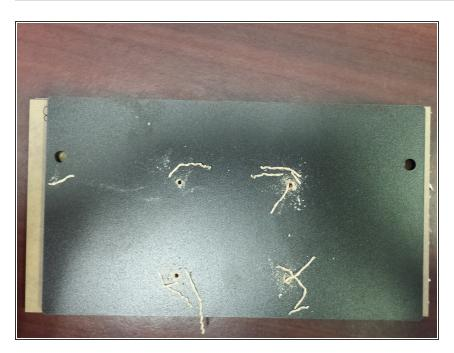
Using a #42 drill bit you should now drill holes in the 4 locations previously marked. Be sure to use a put a scrap piece under the side panel does not split out (and you don't drill through your table!)
