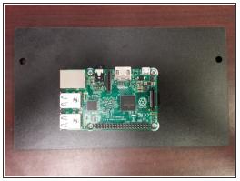
Using the (4) provided standoffs and (4) #4 screws, attach the Raspberry Pi to the side panel. The Micro USB connector should be facing up and the USB and ethernet connectors should be facing to the left of the side panel. Be sure not to over-tighten the screws!
