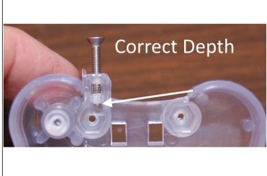
Install one #4-40, 3/8" flat head screw into the top of each inner carriage half. Make sure you drive the screw to the depth indicated in the photograph.
