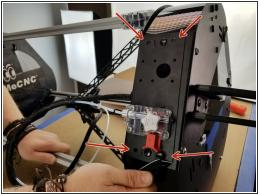
CAREFULLY use a thin object like a screwdriver or pocket knife to pop out all four plastic push rivets that are holding the extruder plate in place.
