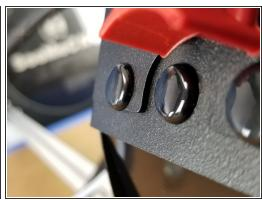
Re-install the plastic rivets by placing them in the mounting holes in the sheet metal, pushing the bottom portion in fully, then pushing the head until the rivet snaps in place flush with the sheet metal.
