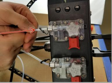
Clip the "C" shaped end of the lanyard into the black ring of the PTC fitting
