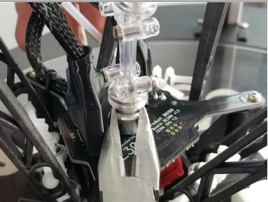
Finger tighten the locking nut, then carefully tighten fully with a pair of pliers.
