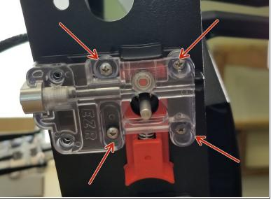
Use the included 30449 M3 - 0.5x 10mm L Phillip Pan Head Machine Screws to attach the EZR Struder and stepper motor to the extruder plate
