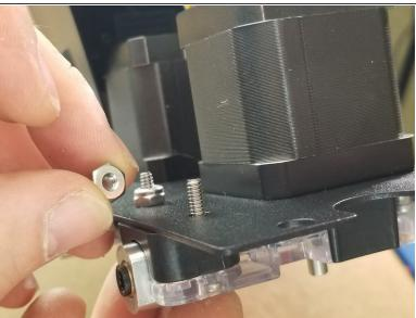
• Use the included 30115 6-32 x 7/8"L Phillip Pan Head Screws and 30164 6-32 Nylon Lock Nuts in the locations shown to fasten the extruder in place, just as the existing extruder is.
