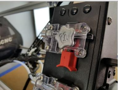
Install your 70714 Stepper Motor 5mm Shaft Handwheel, lining the flat of the hole up with the flat of the motor shaft.
