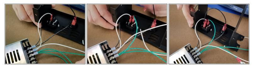
• Take the white wire with spade connector from the power supply and attach it to the leg of the power plug as shown in Pic 1.
