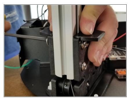
Install the last remaining small shim on the Z tower.
