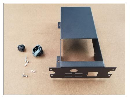
This step we will be assembling the power supply cage. You will use the sheet metal power supply mount, rocker switch, 2x fuses, 2x M3 nylon insert lock nut, 2x m3 x 10mm long phillips screws, and plug receiver with fuse holder
