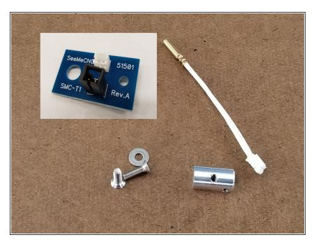
• We will now be prepping the heated bed parts. You will use the cartridge thermistor, aluminum thermistor
