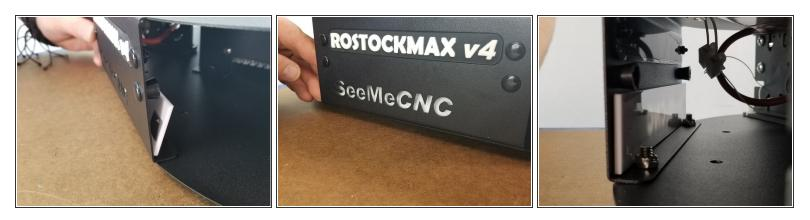
• Line the white acrylic up behind the logo and press the double sided tape into the sheet metal to secure it in place.
