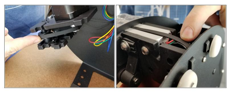
• At this point look at the top and bottom idlers to make sure the belts are seated in the grooves of the idlers properly before clamping in place.
