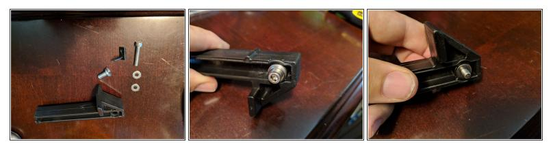
• For this step we will need the Spool hanger (large injection molded plastic piece), Stainless steel insert, Threaded screw and 2 washers.
