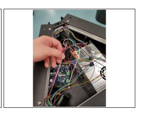
Pull the wires through the tower until the mesh loom enters the hole in the tower and there is enough wire to reach all the connection points in the top assembly when wrapped around the tower.
