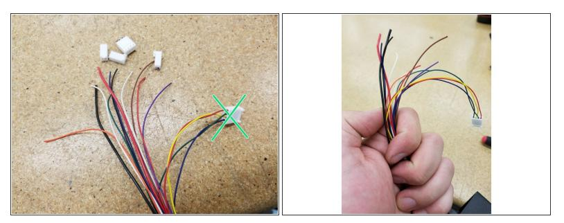
You will need to snip the terminals off the ends of all the wires you unplugged form the Duet. Don't snip the extruder terminal!
