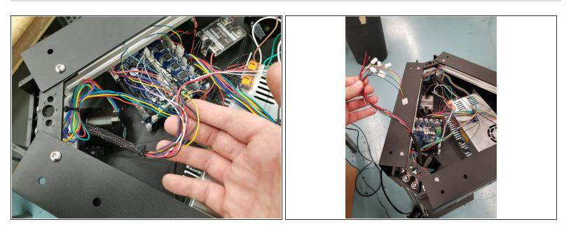
Coming from the X tower, a short section of mesh loom houses the hotend whip wires and the extruder wires. Disconnect all connectors on wires exiting this mesh loom.
