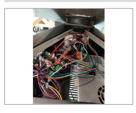
Plug the top cover fan connector back in to place and reinstall the top cover with the push rivets you removed in the beginning steps.
