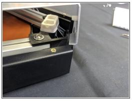
• To remove the cover, lift it straight up on all three corners. You will then need to gently pull out on the silver sides (one corner at a time) to un-hook the cover.
