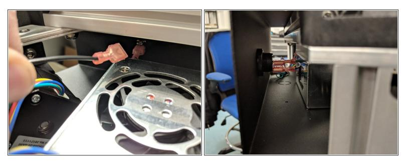
• The power switch connector (black wire with spade crimp, exiting the Z tower wire bundle) connects to the free tab on the power switch as shown.
