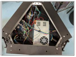
The brown wire exiting the Z tower with NO connector on it will install in the only empty clamp on the relay.
