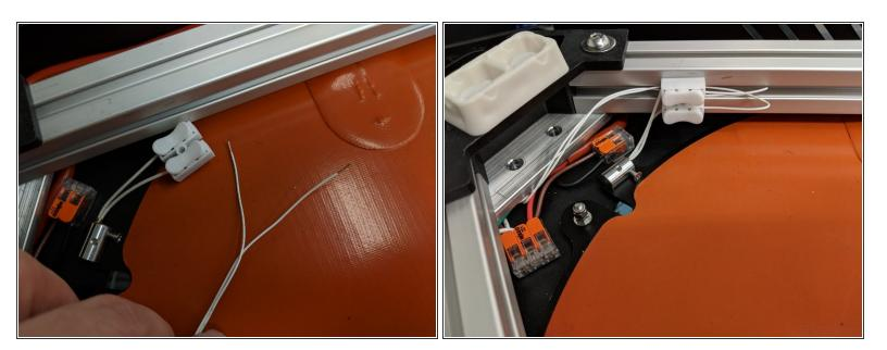
Your final two white 26awg wires exiting the Z tower in the bottom assembly will connect to the white toggle connector as shown.
