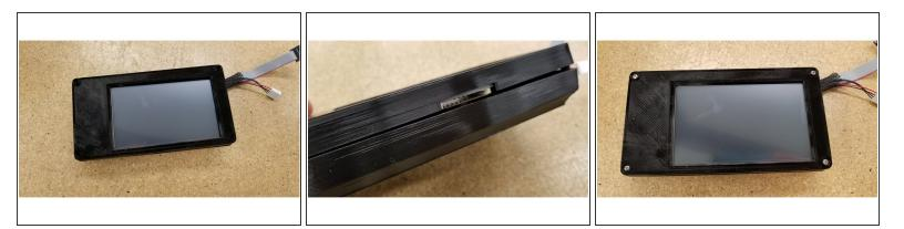
• Align the front half of the screen enclosure as seen.
