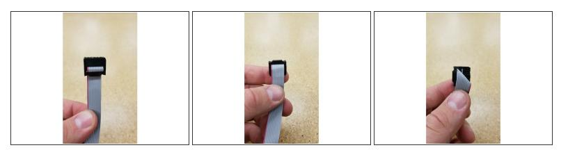
• Hold the loose end of the ribbon cable and fold it exactly as shown in photos 1, 2, and 3.
