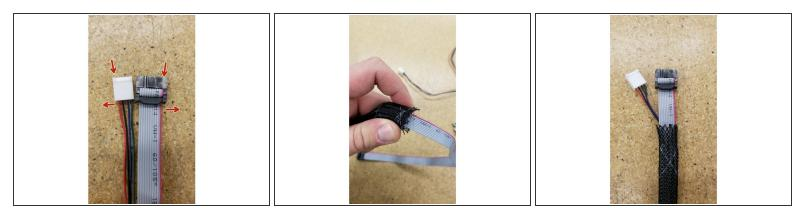
Please note that the 4 pin molex connector is no longer included with the kit. Only use the ribbon cable as the 4 pin cable is no longer used.
