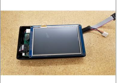
Pass the cables through the hole in the back of the enclosure, and insert the screen as shown.
