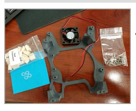
Printed Duet Standoff. For this step you will need the 40mm fan you previously removed from under the Rambo, your 3D printed Duet standoff, the small hardware bag containing 10 screws, and the 4 Nylon washers from the Duet Connectors bag located in your Duet WiFi box.
