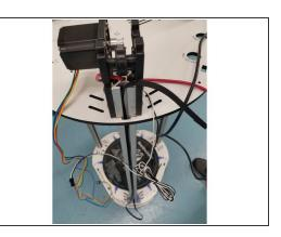
The Next step is removing the top belt clamps from the carriages. To do this take a flat head screw driver and wedge it under the Belt Tension Clamp. Once you have the flat under the clamp you want to give it a counter clockwise quarter turn until the clamp pops free of the carriage.
