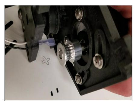
This video shows what your stepper motor should look like with new timing pulley installed and also shows the range of motion you should have for belt tension later in the guide.
