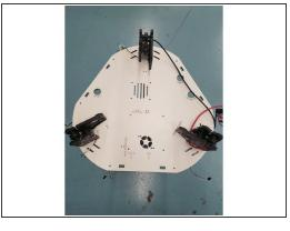
Next step is removing the Timing pulleys from the stepper motor. To do this you will need a 2mm Allen wrench. Loosen the two set screws on each Timing pulley until they are backed out enough to pull the Timing Pulley off the stepper shaft. Do this on all the 3 motors
