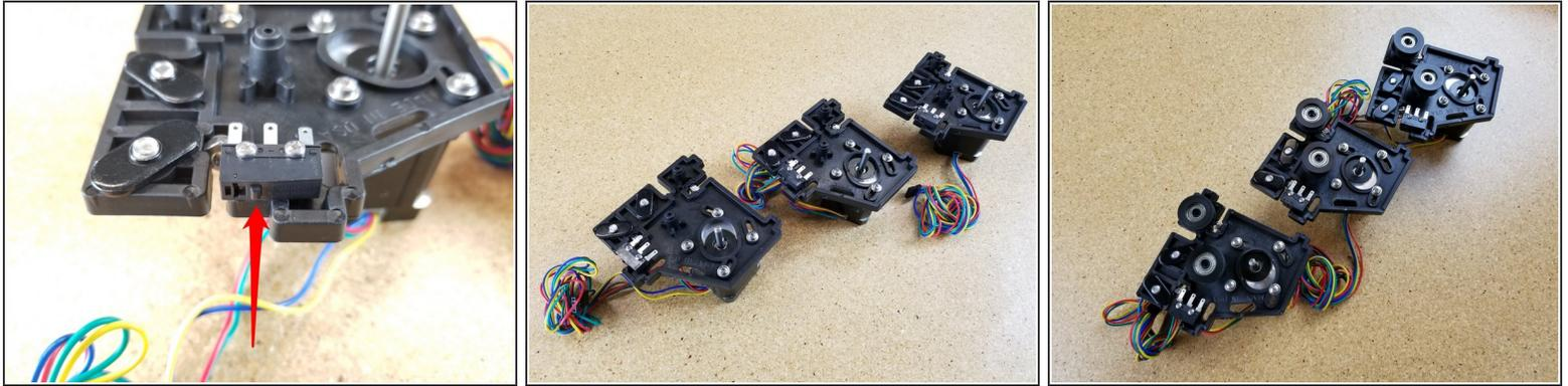
**⚠** When installing the end stop switches, please make sure that they're oriented as shown in the photos. (The red arrow is indicating the "button" on the switch. It should be closest to the T SLOT hardware. Additionally, make sure that the endstop switches are level. This can best be done by pushing them up or down as you tighten the screws.
