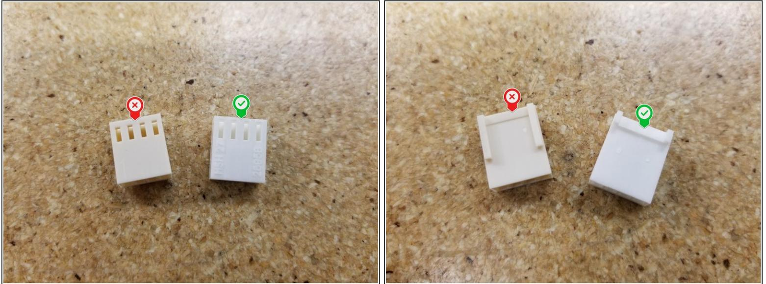
**⚠** When inserting the wires in the white Molex KK connectors, make sure you're using the connectors we sent you in the kit, NOT the ones included in the Duet box!
