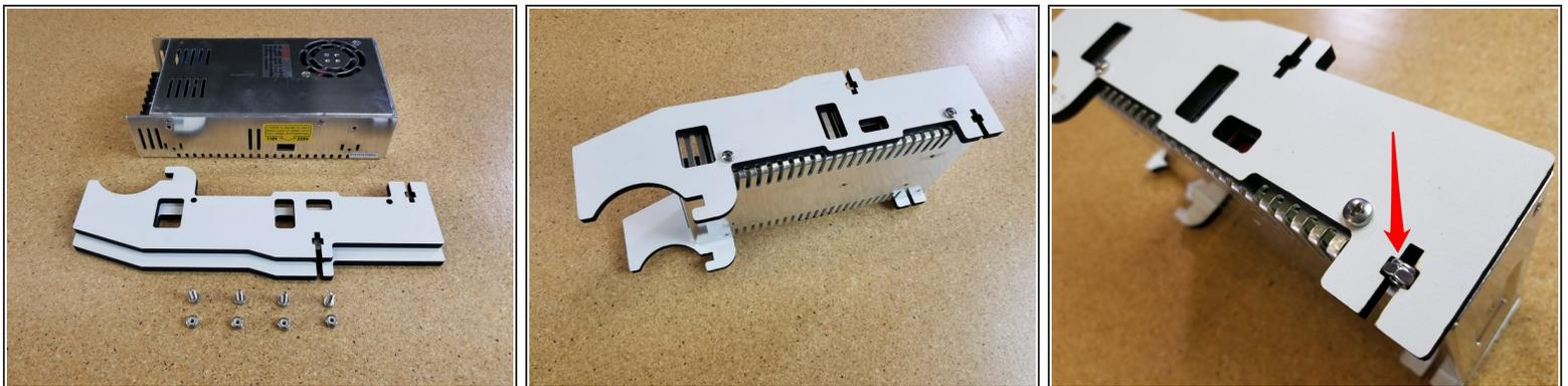
**⚠** If your kit came with screws longer than 12mm, [please email us a support ticket](#). Some kits were packed incorrectly Feb to June 2018 with 16mm long screws. These will damage your power supply. We will ship replacement at no cost.
