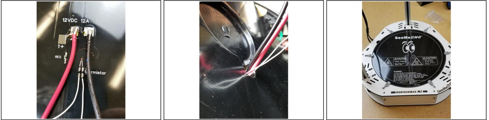
**⚠ Be sure to pass the bed wires through the black injection molded insulator BEFORE soldering the wires to the bed!**
